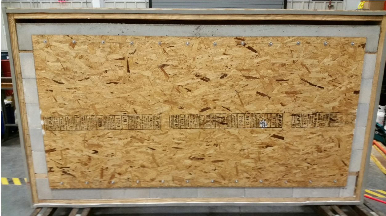
Figure 7. Configuration C1 (with structural wood panel installed)
