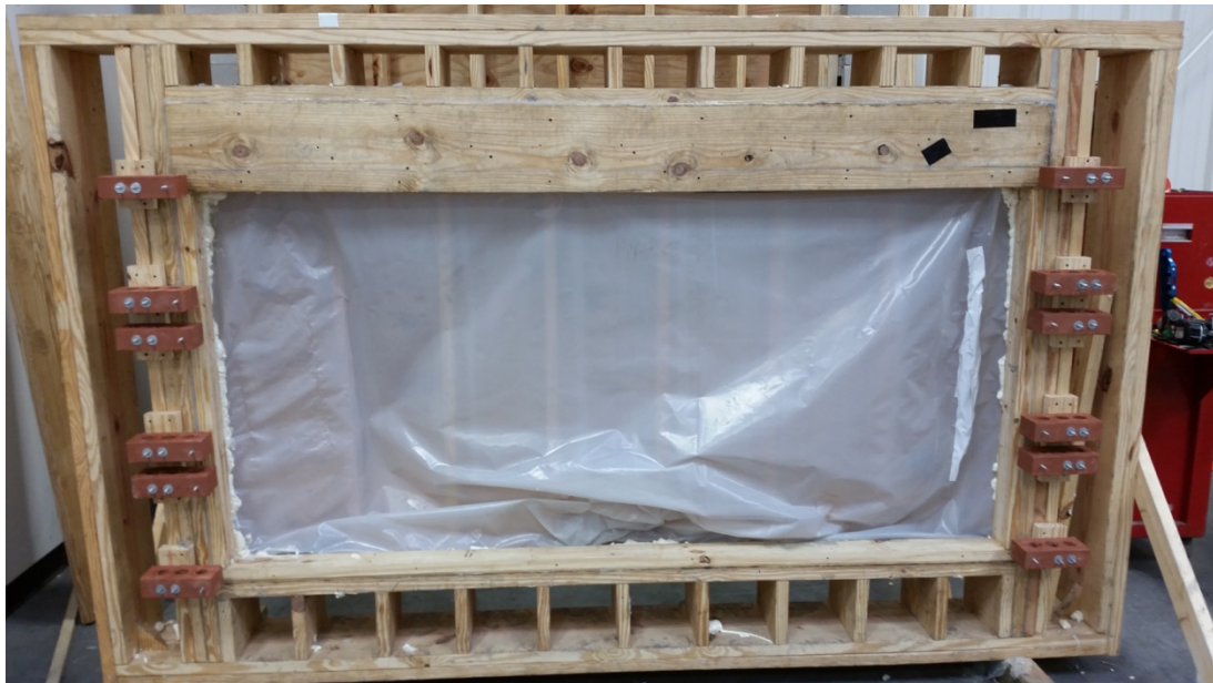
Figure 11. Configuration B2 (without structural wood panel and perimeter blocking to seal the ends and edges)
