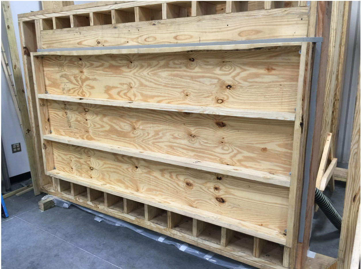
Figure 9. Configuration W2 (with structural wood panel installed)
